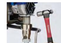
1) Loosen the clamping nut
