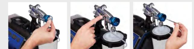
1) Remove front air cap and nozzle
